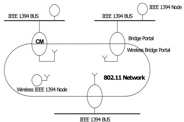
Figure 1. IEEE 802.11 network connecting bridge and non-bridge 1394 devices
