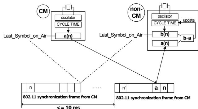
Figure 2. Multimedia Clock Synchronization principle
