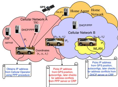
Figure 2: GPS-IP fast-handoff scenario
