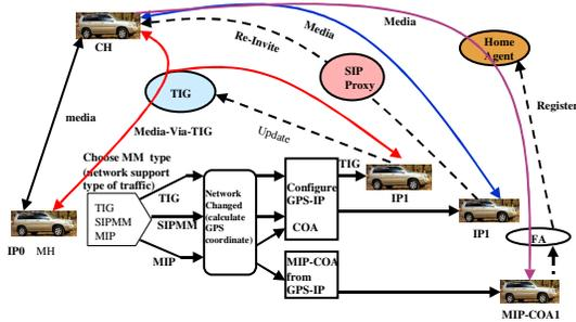
Figure 4: GPS-IP enabled Mobility Management
