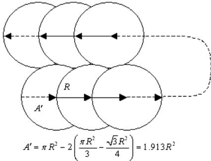
Fig. 1. Upper-bound efficiency of flooding
